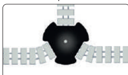
KBK Switch Junction box for networks with up to 3 connection points
